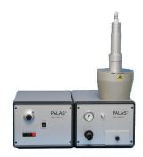
Generation of test aerosols from powder, dust, pollen, etc.; mass flow approx. 8 g/h to 6 kg/h.
