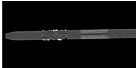
sagittal view: X-ray image of phantom with stent attached
