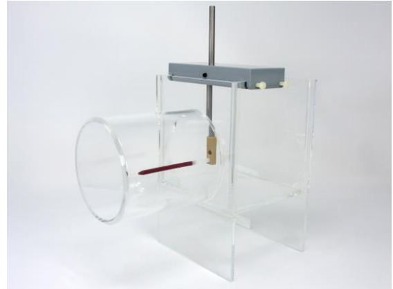
Static holder with coronary artery phantom in Water Tank (Holder: QRM-60109; Water Tank: QRM-10113)
