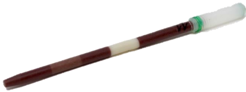
coronary artery phantom with two different circular stenosis
